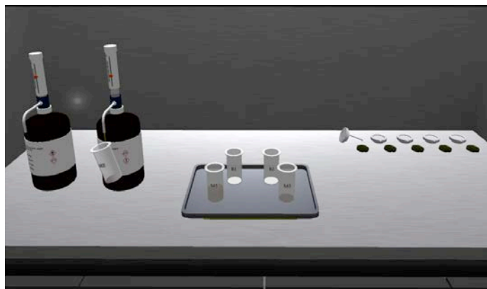
Figure 7. In a hood in Room 2: Hoods, the avatar adds the corresponding digestion mixtures to the vessels, closes them with the Teflon tops and puts on them the safety valves.
