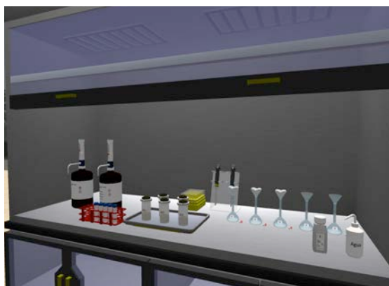
Figure 9. After sample digestion, the avatar comes back to Room 2: Hoods to open the microwave vessels and filter the samples, add the internal standard and dilute the samples up to the final volume.
