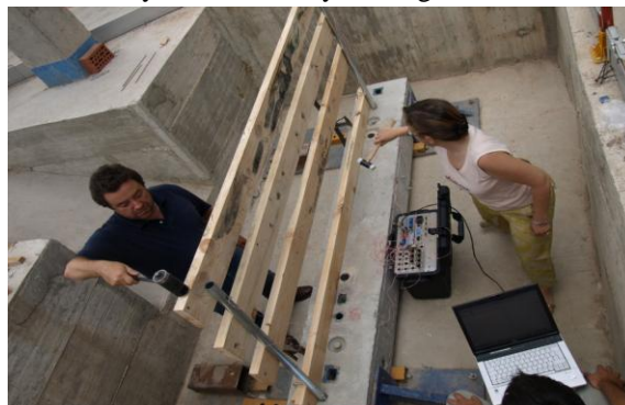
Fig. 6: The process of recording vibrations through random blows with plastic hammers.
