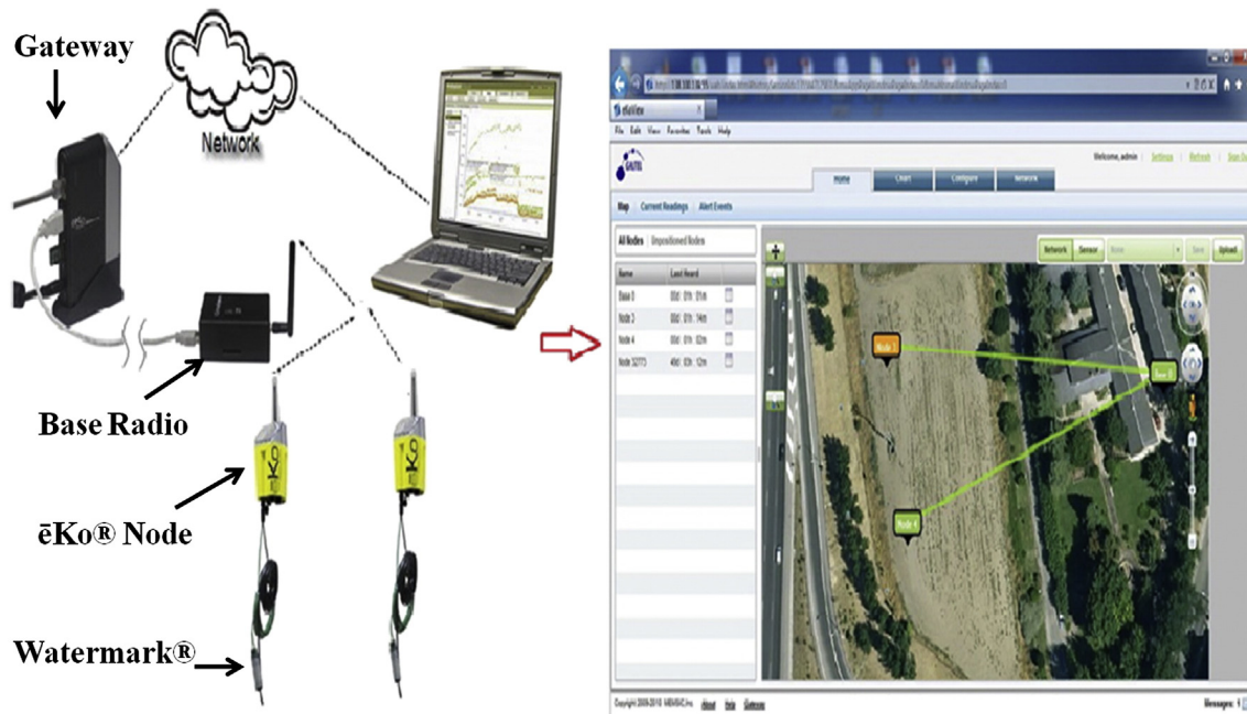
Fig. 1. Scheme for the wireless sensors network components and the nodes deployment in the experimental site.
