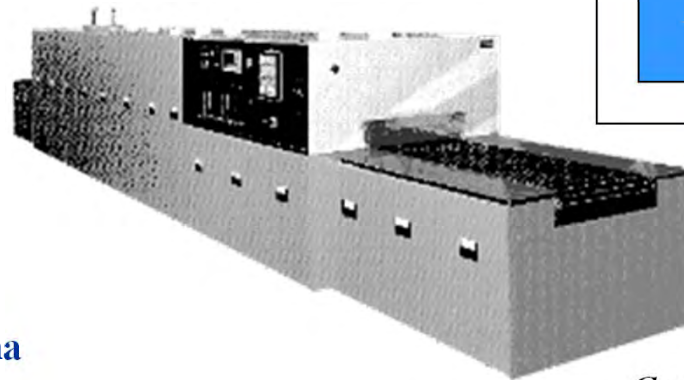
In-line furnace for firing
