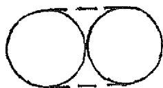
Fig.7. Minimum-perimeter convex envelope (dashed and half-circle segments) for a cross-section made of two adjoining circles.
