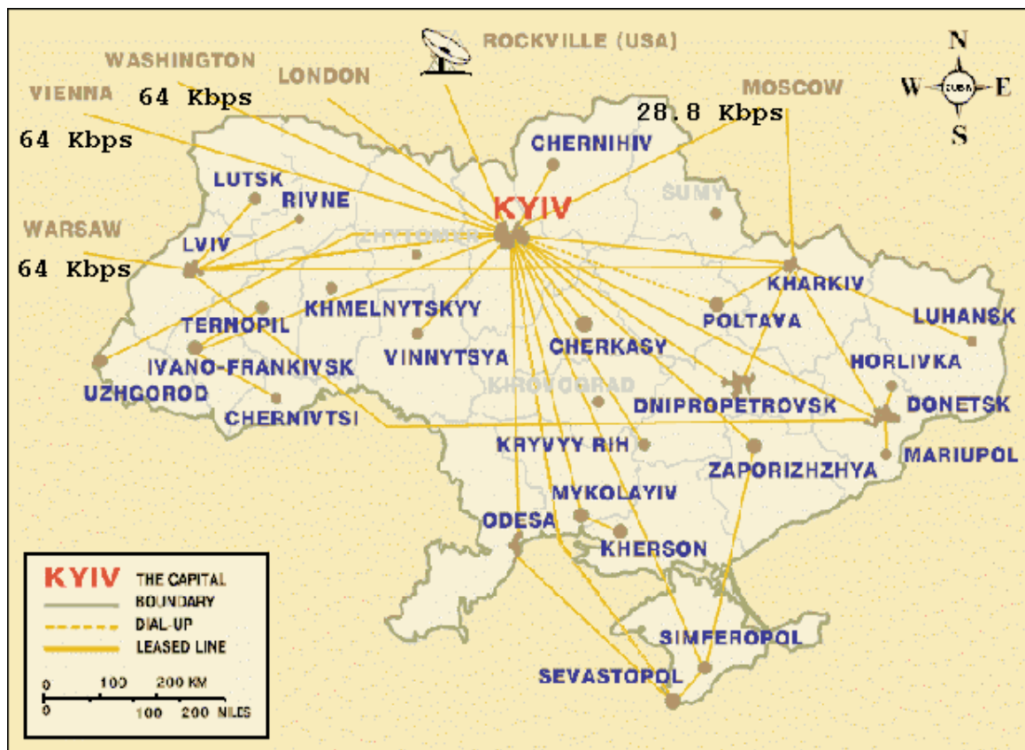
Figure 8: Structure of a telecommunication network of Ukraine.
