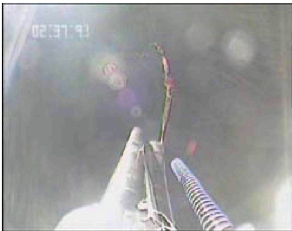
Fig.2 Bare electrodynamic tape tether deployment on S520-25 [Courtesy of ISAS/JAXA, Left: Seen from MOT (Mother) Rocket Time X+158sec (Tether is in the jumping rope mode.), Right: Seen from DAU (Daughter) Satellite]
