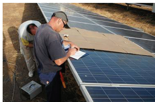
Figure 9: Cardboard covering the area of a module which is being biased with a current source (lower left corner).
