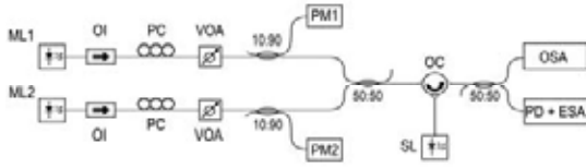
Fig. 1: All-fiber experimental setup: (OI) optical isolator, (PC) polarization controller, (VOA) variable optical attenuator, (PM) power meter, (OC) optical circulator, (OSA) optical spectrum analyzer, and (ESA) electrical spectrum analyzer.
