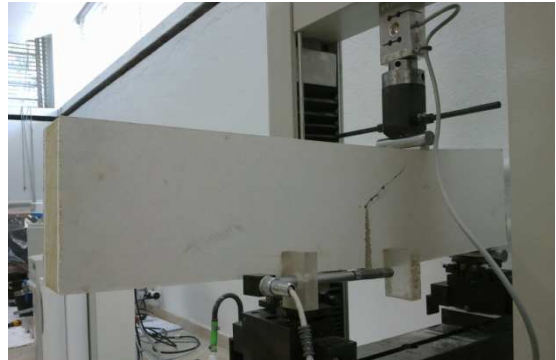
Figure 6: Sandwich panel specimen, under mixed mode fracture testing. Specimen of 150 mm height.
