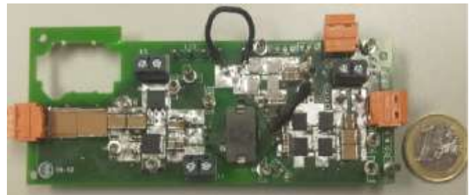
Figure 10. Photo of the three port bidirectional 300W 700 kHz prototype.
