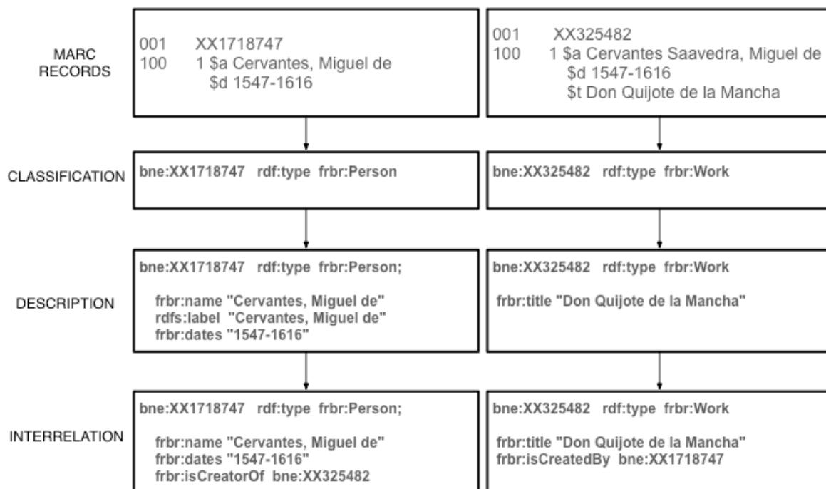
Fig. 5. An overview of a mapping process for authority records ( RDF statements in Turtle serialization )
