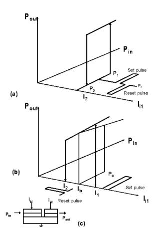
**Fig. 11.-** (a) (b) Bistable laser diode characteristics (c) Laser diode structure.
