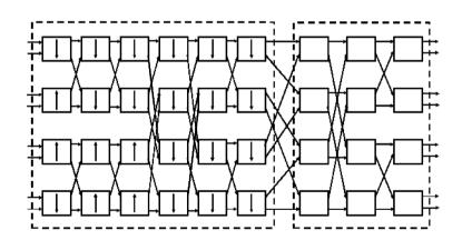
Fig. 10.- An 8 x 8 Batcher – Banyan structure.
