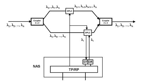
**Fig. 3.-** Proposed OADM using parallel architecture with optical programmable logic cells and fixed-wavelength transponders. OT and OR correspond to Optical Transmitter and Receptor. NAS is the Network Access Station. TP/RP stands for Transmission/Reception Processor.
