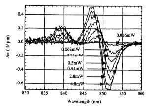
**Fig. 5.-** Spectrum of absorption change measured in a type II hetero-*nipi* containing coupled quantum wells<sup>5</sup>.
