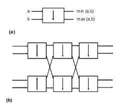
**Fig. 8.-** Basic comparison block in a Batcher Network (a) and definition and a 4 x 4 Batcher switch (b).
