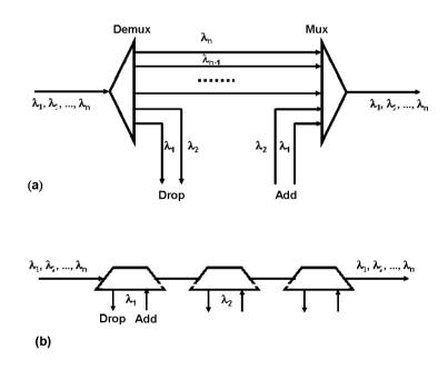
Fig. 1- Optical Add/Drop architectures. (a) Parallel configuration; (b) Serial structure
