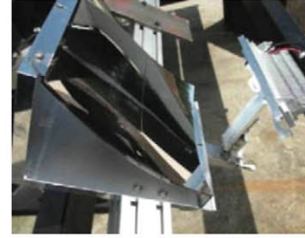
FIGURE 5. Single-cell unit module test rig of the 800× off-axis XR-Köhler CPV module.
