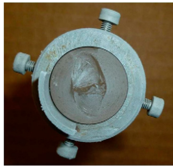
Fig. 7. Failures without fragmentation for a semicircular notch ( R = 6 mm).
