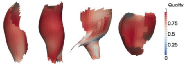
Fig. 3 Results for four representative Abdominal Aortic Aneurysms (AAAs) intraluminal thrombi (ILTs) using the Scaled Jacobian as a measure of element quality.
