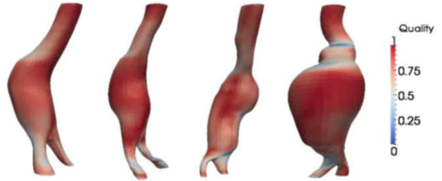
Fig. 2 Results for four representative Abdominal Aortic Aneurysms (AAAs) walls using the Scaled Jacobian as a measure of element quality.
