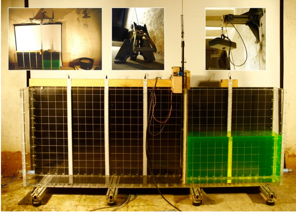
Fig. 1. Experimental setup of the dam-break tests (data acquisition system is not displayed). The imbedded figures display from left to right: the overall setup, the release mechanism, the weight used to induce gate's motion.
