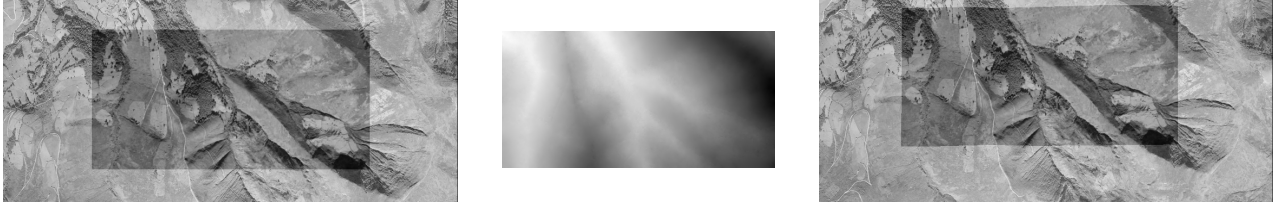
Figure 4. Variational disparity method. Predicted images by transferring intensities according to the correspondence given by the disparity map. Left: original image I_1 (outside the centered rectangle \Omega , with some intensity scaling for visualization purposes) and predicted image \hat{I}_1(\mathbf{x}_1) = I_2(\mathbf{x}_1 + \mathbf{d}(\lambda)) (inside \Omega ). Center: Tangential disparity \lambda(\mathbf{x}_1) , pseudo-colored in grayscale expanding the range of \lambda , in this example \lambda \in [-48.54, -41.11] pixels. Grid size ( \Omega ): 513 \times 257 pixels. Right: predicted image \hat{I}_2(\mathbf{x}_2) = I_1(\mathbf{x}_2 - \mathbf{d}(\lambda)) (matched region) and original image I_2 (outside).
