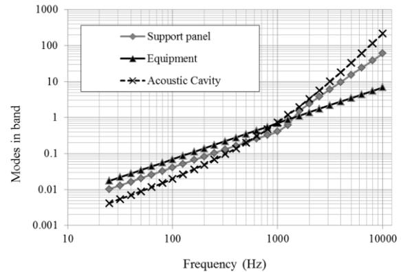
Figure 6. Modes per one-third-octave band of the support panel, the equipment and the acoustic cavity
