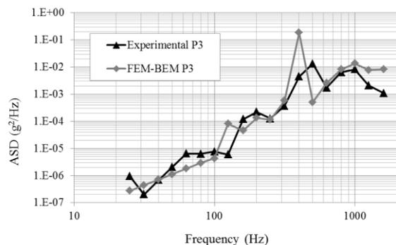
Figure 15. Correlation between P3 simulated and measured acceleration response
