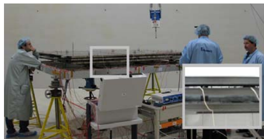
Figure 1. Dutch Space ARA-MKIII solar array in folded configuration. Close up shows the gap thickness between panels.
