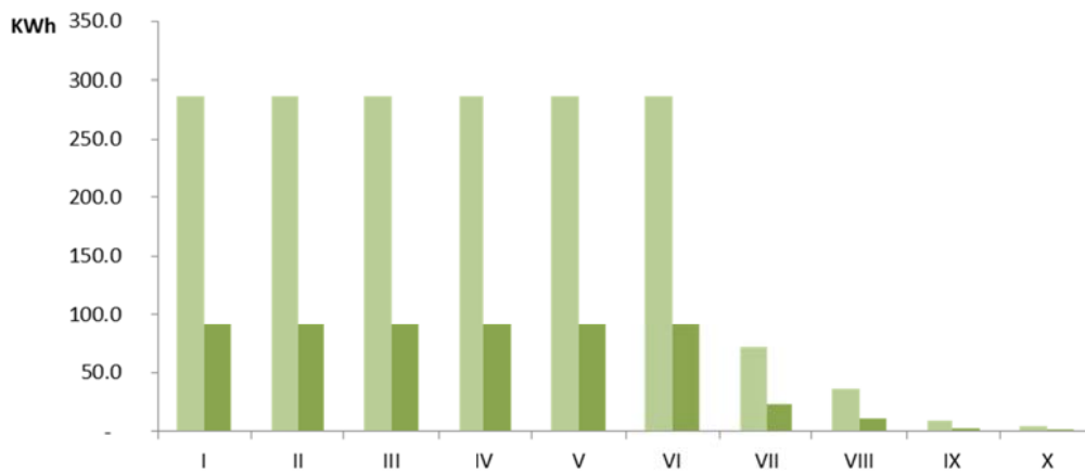
Figure 8.13 – FTTx/VDSL profile of energy consumption per access area for the year 2011
