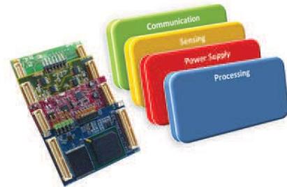
Figure 7 Four layers architecture and physical view of the node
