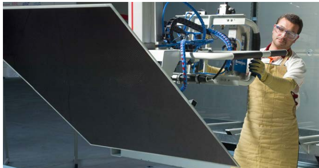
(c) a-Si:H Typical efficiency 7-8% Image: T-Solar
