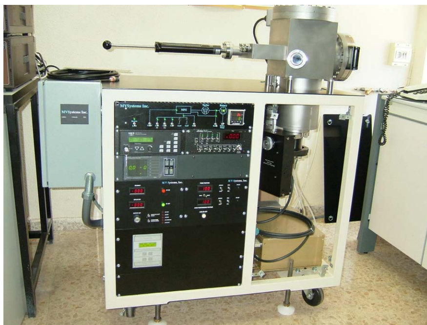
Figure 3.2: RF sputtering plant using a MV Systems device at CIEMAT facilities
