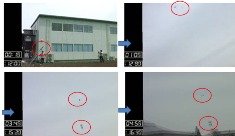
Fig. 7. Tape tether deployment test using a water rocket model.
