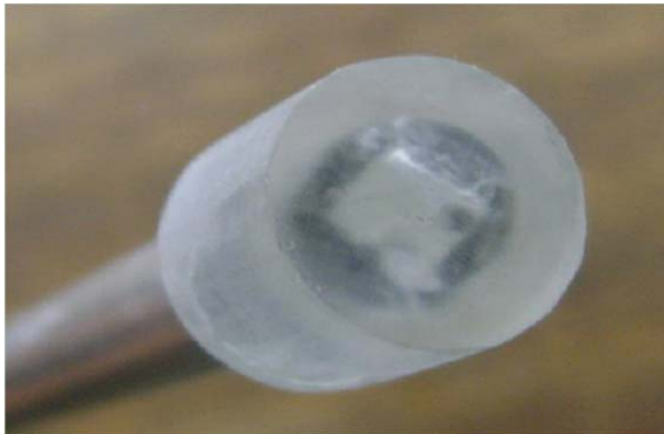
Fig. 2 Rexolite layer mounted on the transducer.
