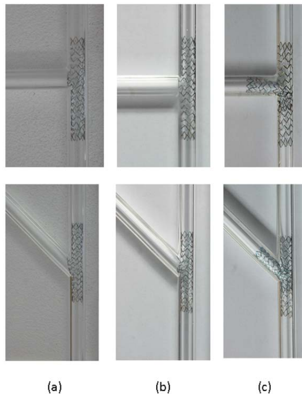
Figure 1. Stenting techniques considered in this study: (a) simple stenting in the main branch, (b) simple stenting with kissing balloon through the side branch and (c) culotte stenting.
