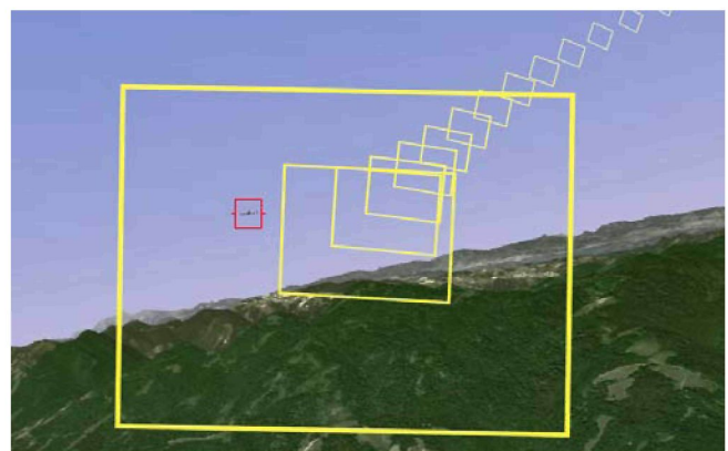
Figure 5. Tunnel-in-the-Sky Synthetic Visualization of the Automatically Generated 4D Trajectories to the Flight Crew
