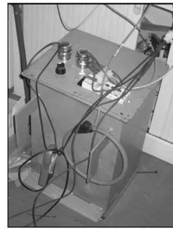
Fig. 9. Voltage stabilizer and regulator prototype.
