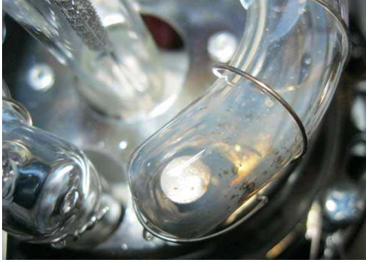
FIGURE 6. Signs of degradation as depositions in the inner side of the bulb near the electrodes.
