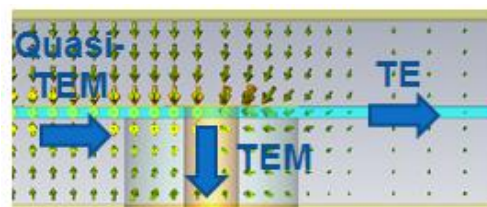
Fig. 3 TE mode generation in vertical transitions
