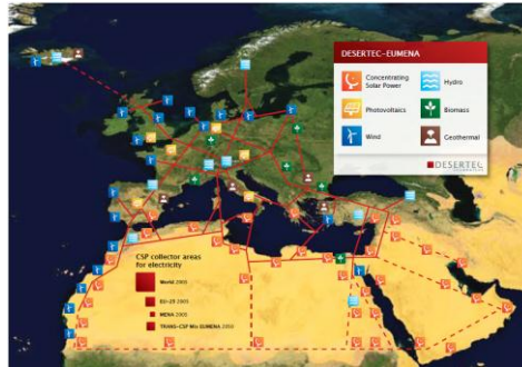
Figure 7: Concept of a „EUMENA Supergrid“ based on HVDC power transmission as “Electricity Highways” to complement the conventional AC electricity grid, as developed by TREC in 2003.
