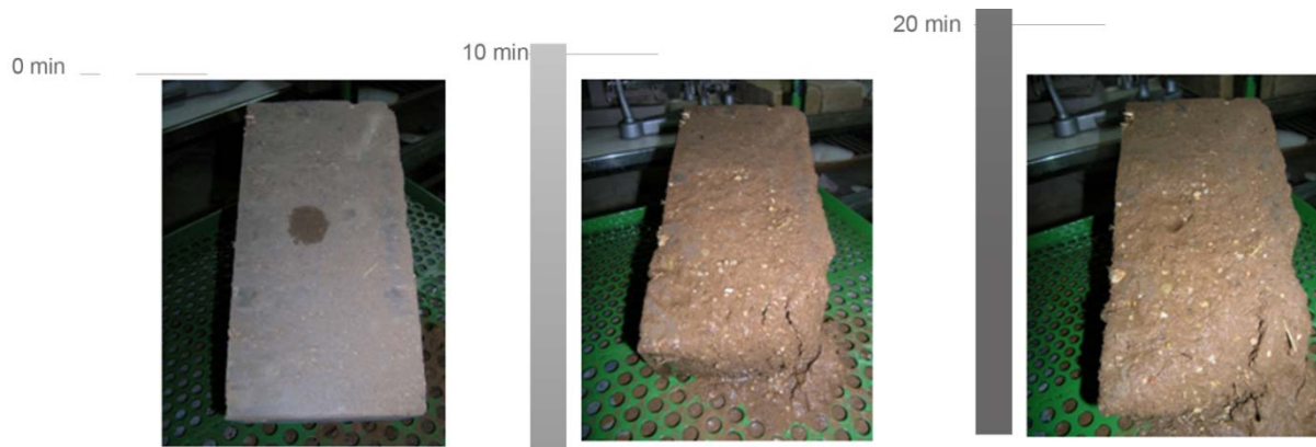
FIGURE 3: Drip erosion test (non-stabilized block )
