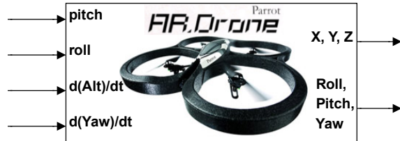
Figure 1: AR Drone black-box model. The specified inputs match the real system's. The euler angles and the altitude outputs are available from the AR Drone telemetry data. To the contrary, the only available data from the drone about the X and Y directions are speed measurements obtained by means of optical flow algorithms.
