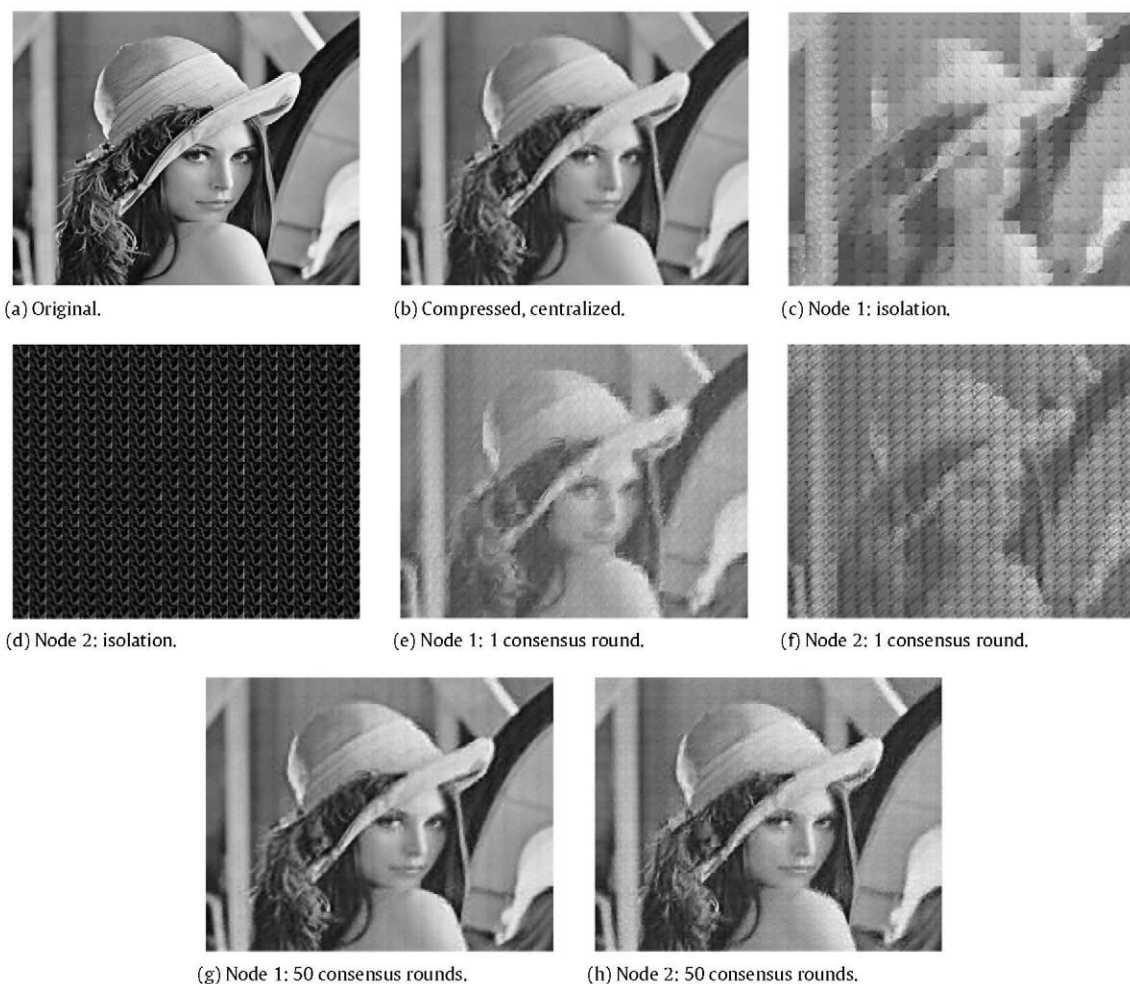
Fig. 5. Performance of PCA in isolation and with cooperation via consensus using CB-DPCA. Images (c), (e), and (g) illustrate how a node asymptotically converges to the centralized solution given in image (b). Images (d), (f), and (h) show the same for another node in the network.
