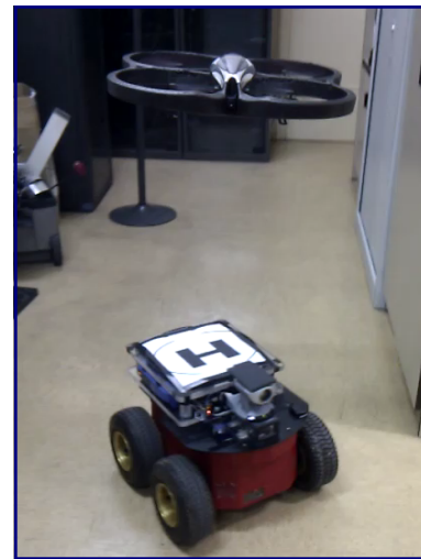
Fig. 8: First communication and hovering tests - The UAV - UGV communication capability when performing hovering over the UGV was successfully tested.
