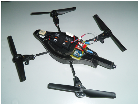
Fig. 3: UAV with external GPS system.
