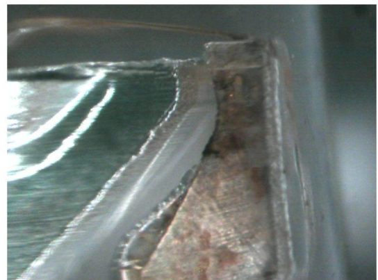
Fig. 9. Anode oxidation due humidity penetration.
