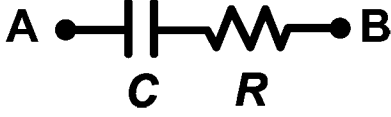
Fig. 8. Simple RC network that is used to present each branch of the implemented analog multiplexer.
