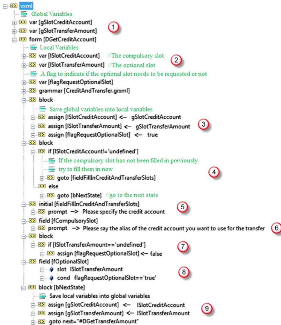
Fig. 7. Example of VoiceXML generated for a dialog with over-answering.
