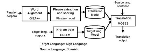
Figure 7. Diagram of the phrase-based translation module
