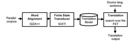
Figure 8. Diagram of the FST-based translation module
