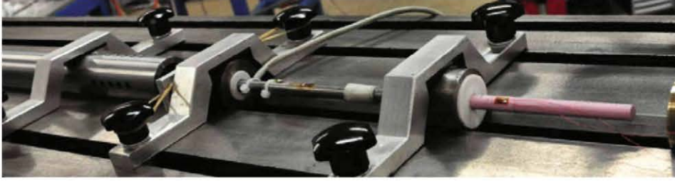
Fig. 3. Experimental set-up showing the barrel, the incident bar, the instrumented specimen and the fragment recovery system. All items mounted over a V-shape bedplate.
