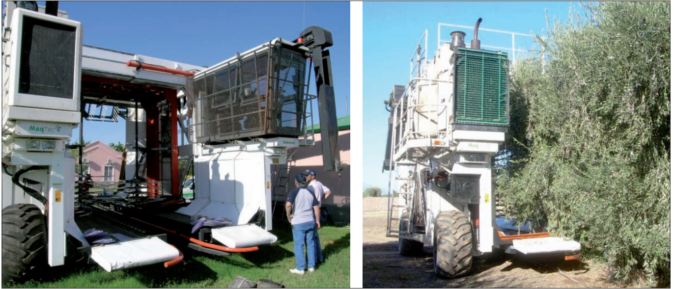
Photo 17. Over-the-row harvester (Colossus) for harvesting oil-variant olives, which can harvest trees up to 4 m high and 4m wide.
