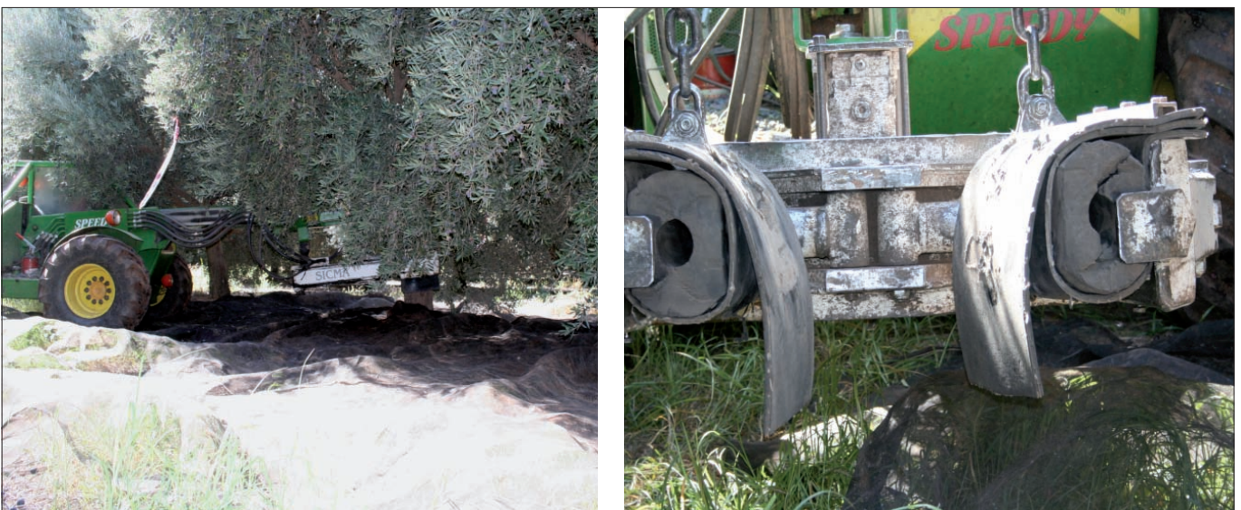
Photo 16. Trunk shaker for harvesting oil-olives. This is being used with success even in large trees (up to 5 m in height), provided they have been properly pruned to allow transmission of the vibrations.
