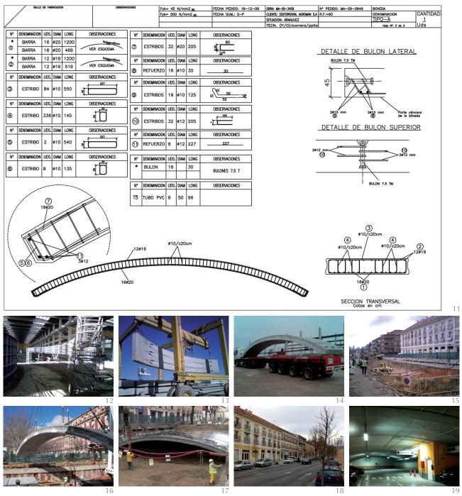
Because the elements have been concreted in a vertical way the elements have to be tilted to the final horizontal way. The tilting has to be done in the factory with the help of large mobile cranes (Figure 13).
