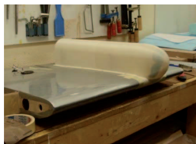
Figure 11. Fairing, placed and fixed onto the wing
