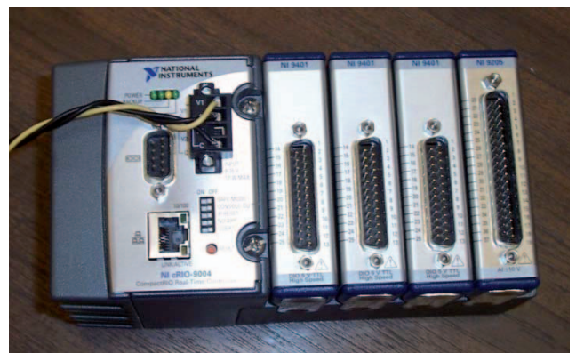
Figure 14. CompactRIO® 9004, with 4 modules
