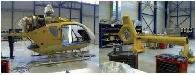
Figure 7. Different phases (b) of the mounting process of an helicopter. Copyright: the authors. Licenced by Eurocopter, an EADS Company.
