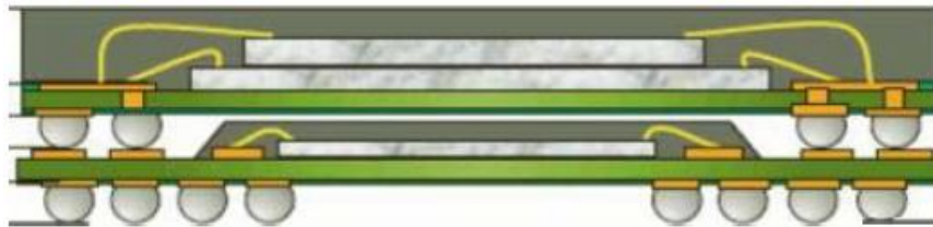
Fig 28: Encapsulation and POP type structure of the OMAP35XX processor.
