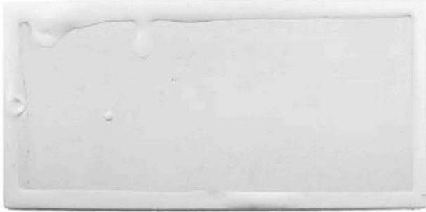
Fig. 7. GPS Al slurry coating painted with chromate-free epoxy primer after immersion in water for 168 h followed by tape application and removal (ASTM D 3359).
