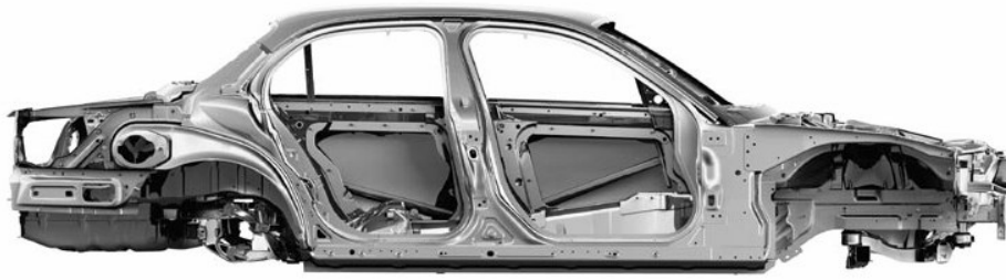
Figure 2: An illustration of the aluminium body structure of the Jaguar XJ that is constructed of aluminium alloy extrusions, sheet pressings and castings joined together by self-piercing rivets and adhesives. (Picture courtesy of Jaguar)
