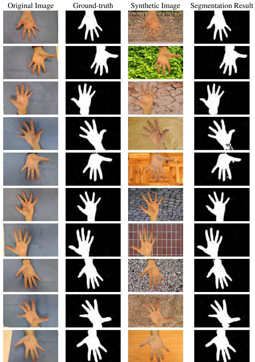
Figure 3: A comparative study of results provided by segmentation algorithm in comparison to ground-truth. First column gathers examples from first database, together with their segmentation on second column, considered as ground truth. Third column presents synthetic images based on first column images, providing on the fourth column the final segmentation result.
