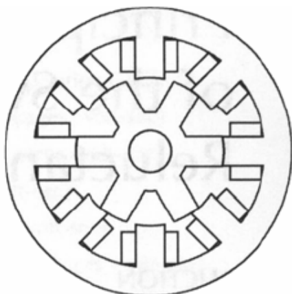
Fig. 2. SRM Geometry: 4-phase, 8 rotor poles/6 stator poles
