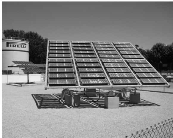
FIGURE 3 6.5kWp Pirelli Pilot Plant in Manresa (Spain). The tracker holds 40 panels comprising 48 Köhler lenses and cells each. Picture courtesy of Pirelli.
